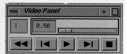
FIGURE 6 Video panel tool for seismic wave propagation animation. It provides stop-start and frame-by-frame stepping functionality to the animation.
