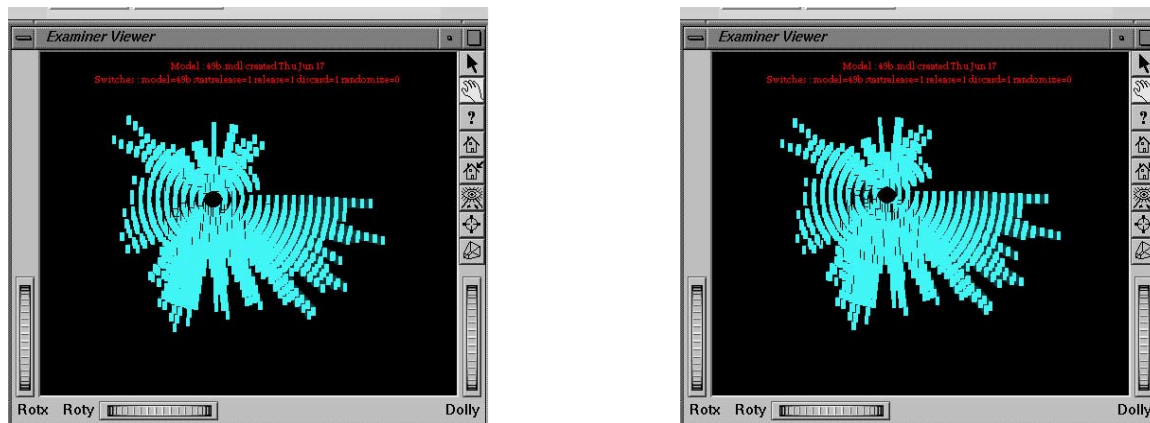
Figure 5. Platter Metaphor: Route Distribution. The left (A) and right (B) images show two different algorithms for route configuration. The difference between these networks is minimal and this indicates little difference in number of routes in an OD pair for both configurations.
